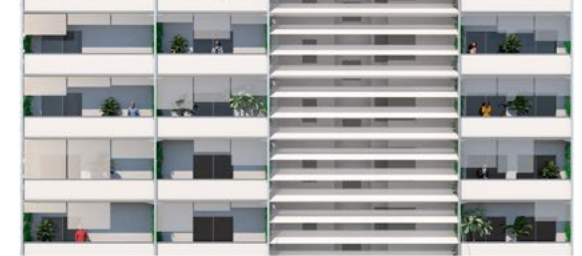
B: The balcony increases indoor ventilation and lighting, and curtains are hung on the east side for sun protection.
