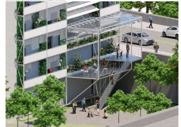
E: Photovoltaic roof stores electricity to provide balcony lighting and reduce rooftop sun exposure.
